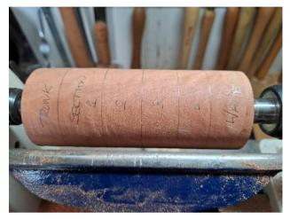
1. Start with a blank (between centres) around 50mm wide, by 150mm long, and turn to round. Once you have it round Mark out the sections of the tree with the base/trunk section at the headstock end, and the tree sections toward the tailstock. Mark each tree section a little smaller than the last, to accommodate the narrowing of the tree as it reaches the top. You're aiming for five (or more) sections above the trunk, with the last being waste.
