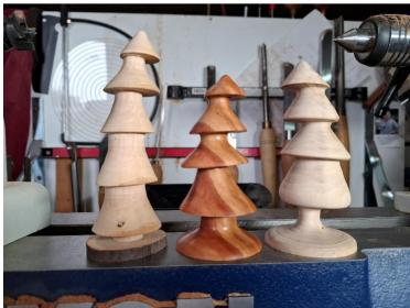
7. Part off the top and hand sand the very point. The base can be hand sanded, but should a linisher be available, it's a lot quicker. The two pictured without any finish were turned from branch timber.
