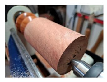
5. Move the tailstock centre to position 2, and repeat step 4. This process then repeats as you work your way up the tree.
