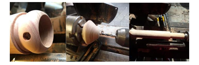
Turn the outer shape of your ring. The hole is longer so the ring should come off as you finish shape.
