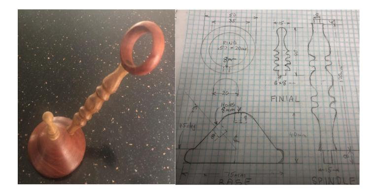
To make a turned bottle holder stand you require a piece of timber 100 \* 75mm for the base and ring.
