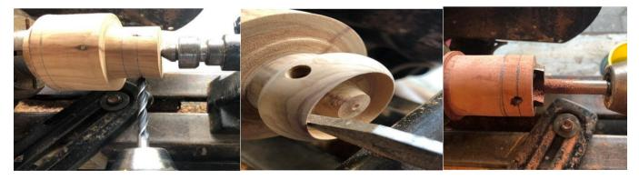
Spindle turn the 100 \* 75 to round 75mm.
