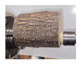
Using a cone live centre in your tail stock, bring it up into the hole for support. A small amount of masking tape around the coned will prevent it marking the wood. Shape the trumpet section of the holder and sand when complete.
