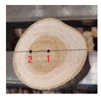
Begin by marking centre (point 1) on both ends of your blank and drawing a line through the centre point. Ensure that the line is the same direction on both ends. Mark a second point along the line (point 2) on both ends. Ensure that the second point is the same distance and direction away from centre on both ends. This will be your offset. The distance used in the picture is 20mm. Mark the points with an awl.
