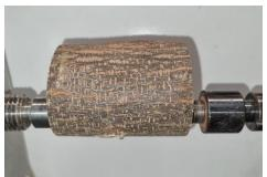
Mount between centres on the offset points and turn a tenon on one end of your blank to suit your chuck. As your blank is well out of balance a slower lathe speed may be needed.
