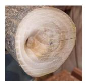
Once your hole is drilled, flare out the end of the hole to make the inside of the trumpet part of your pen holder. Sand when completed.
