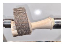
Remove your masterpiece from the chuck and remount between centres using a cone live centre and your favourite drive centre, using the actual centre (point 1) marked at the start on the base.
