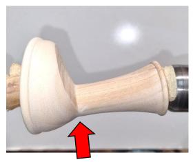
Shape the base section of your pen holder. Take care not to cut into the section of the trumpet indicated by the red arrow. This usually involves stopping the lathe a few times to be sure. Sand when completed. Having your sand paper wrapped around a soft rubber block will make it much easier and less damaging to your fingers. Part off carefully once completed.
