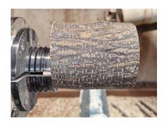
Mount your blank into your chuck. Next with a drill in your tail stock, drill a hole for your pen. The hole only needs to be 40mm – 50mm deep. The drill pictured is 10mm
