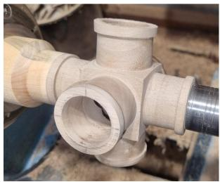
**11.** Using carving tools (hand or powered), files or rasps remove the square centre sections and sand to complete.
