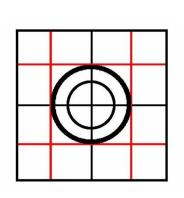
Measuring with a ruler or using a carpenter's square, draw lines parallel to the edges of your blank and to the edge of your larger circle. These lines are the most important, so ensure they are quite dark. Repeat on all 6 faces.
