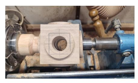
8. Using the 'important' lines marked earlier as a guide, turn down the side of your blank to the jamb chuck. Work slowly as cutting past these lines will remove timber from your 'pipe wall'. Repeat on all 6 sides.
