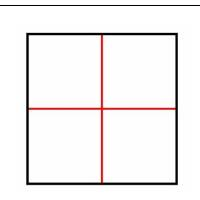
Begin by marking the centre of each face of your blank. Using an awl or similar, mark the centre point as accurately as possible
