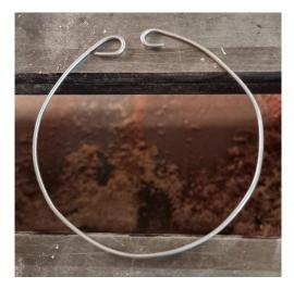
This is a home made feeler gauge made from a piece of wire. Note that the ends have been turned in to prevent scratching of the bell.
