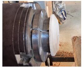
Do not discard the stub left behind after parting off. This stub now becomes the jam chuck for final finishing of the top of the bell.
