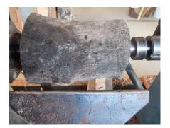
Locate and mark the centres of both ends of your blank with an awl or other suitable device.
