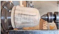
Reverse the bell over the jam chuck and align using a cone live centre in the hole drilled previously. Take fine cuts to complete the top of the bell.
