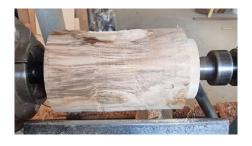
Use a spindle roughing gouge, bowl gouge (or skew chisel depending on your preference and/or skill level) to turn down to round.
