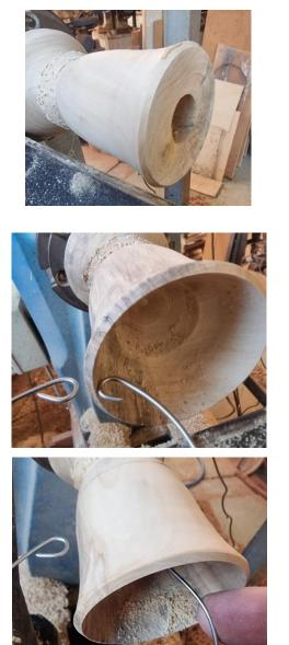
Use a Forstner/saw tooth bit in a Jacobs chuck or other suitable hollowing technique to remove the bulk of the waste.
