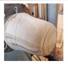
Sand the top of the bell. Tailstock support can be withdrawn for the final sanding of the centre of the top as long as light pressure is applied and directed toward the headstock.
