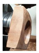
6. Remove the lid section from the chuck and mount the base section using the recessed tenon. Turn a short tenon on the base to accommodate the hollow on the lid section. At this stage make the tenon a tight fit to act as a jamb chuck.
