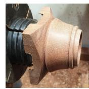
10. Using a scrap block mounted in your chuck turn a jamb chuck to reverse mount the base section. Use the tail centre to hold the base onto the jamb chuck (not pictured)
