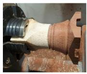
11. Shape the base and feet, taking care not to break the corners of the feet, remove the tail stock to complete the centre area. Sand as required.
