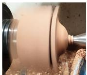
8. Remove the tail stock and very gently complete the centre of the box lid as not to break it from the jamb chuck. Gently sand as required. Once complete, remove the lid from the jamb chuck. If the lid is a tight fit it is advisable to use a knife and gently prise it loose as the corners can be fragile at this point.
