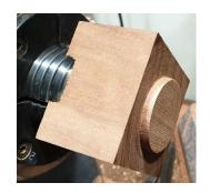
7. Mount the lid section on the tenon (jamb chuck) and using a live centre in your tail stock gently push the lid on to the base to hold it in place. Shape the top of the lid as desired.
