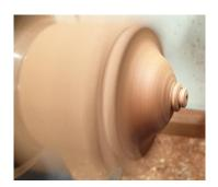
9. Shape and hollow the base section and sand as required. At this stage it is advisable to sand the tenon that the lid sits on to make a slightly loose fit. When removing the lid people tend to hold the lid corners and having a tight or press fit may result in breakage. Remove from the chuck
