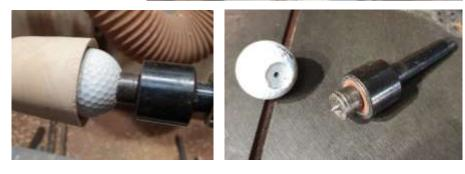
8. With the tail stock <u>gently</u> pushed up, finish the shaping of the outside of the bowl section.
