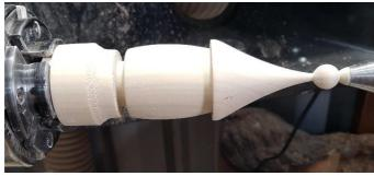
Sand and polish at this point with tailstock support.
