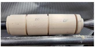
Mark your blank as shown, allow 10mm waste tailstock end, then mark 10mm (for the ball on the hat ) then 65mm ( hat ) and 50mm ( body). The remaining timber will become his nose. Using a parting tool (about 3mm is best) make a cut as shown above to define the parts. Do not cut too deep at the far left (bottom of body) as you need to maintain stability while turning. Timber can now be mounted in the chuck but continue to use the tailstock for support.
