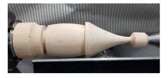
Start by shaping the hat. Then apply some body shape. The hat rim is slightly undercut, this allows the upper edge of the hair to be hidden.
