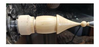
Remove tailstock and gently finish cutting ball, then sand and polish.
