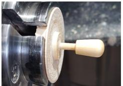
Reduce the remaining timber to approx. 15mm diameter. Now shape and sand the nose.
