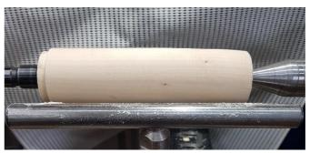
Choose a piece timber approx. 55mm square and 180mm long. Mount between centers and rough down to approx. 50mm diameter. Make a tenon for your chuck on one end. This blank will make the gonk and his nose.
