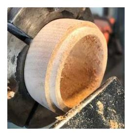
Part off a section approximately 50 mm long. Mount in your scroll chuck and create a jointing tenon before hollowing out the interior.
