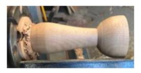
Shape the rattle section to match your hollow or design of your choice. Remember to make the walls thin enough that the sound will transmit through them without being so thin that they are likely to break.
