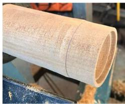
Mount the main section in your scroll chuck. Create the other half of your joint — note: go slowly to create a press fit, you do not want the joint to be sloppy or so tight that you have difficulty separating the sections.
