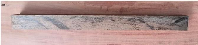
The blank size is up to the individual, but to begin with, try a spindle blank of straight grained wood of approximately 25 mm square and 250 to 300 mm long.
