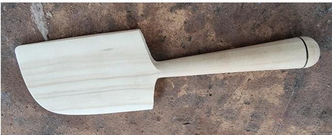
Use a skew or spindle gouge to turn the handle to round. The diameter of the handle where it meets the blade should be less than a mm less than the maximum thickness of the blade.
