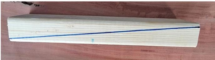
Mark points 4 mm from the opposite edges of the narrow face of the blank and draw a line to connect them as shown in the adjacent photograph.
