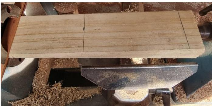
Accurately mark the centre of the thickest end of the blank. Use two pieces of scrap timber to protect the thin end of the blank and mount with the thin end centred in a suitable chuck and the thick end at the tailstock supported by a live centre.
