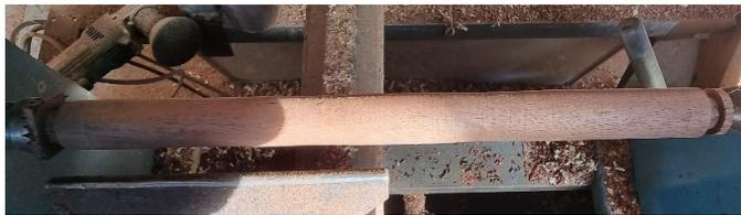
Use a parting tool to form a groove approximately 5 to 10 mm from each end of the blank. Diameter is not important as long as the groove is down to round.
