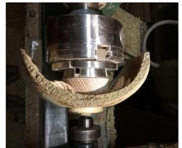
Sand the bottom but again take care working on the wings, which are best done with lathe stopped. Apply finish of choice to the whole piece.
