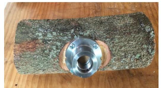
An alternative approach is to remove some bark with a Forstner bit or angle driver, sufficient to attach a faceplate. Turn the tenon on the opposite side. To ensure there is an even thickness and width of bark around the edge line up the faceplate so it is parallel with an imaginary line across the timber.
