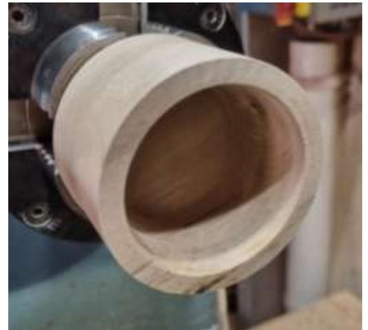
5. Remove your box from your chuck and mount the lid using the recess. Turn down a tenon to suit the inside of your box and tidy the underside of the lid, sand when complete.
