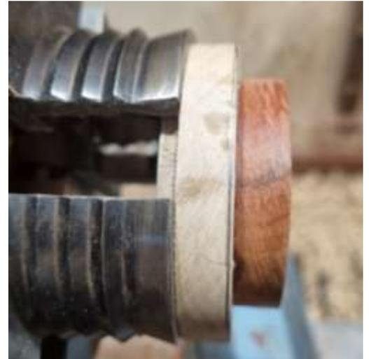
10. Gently turn down the inlay to blend into the lid. Sand when completed and finish as desired.
