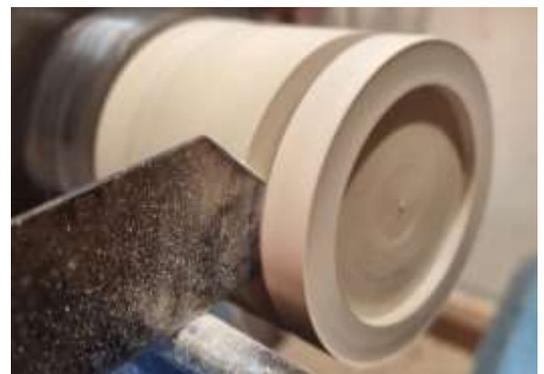
4. Mark the wall thickness of your box – leaving it slightly thicker than your desired finished size and hollow. Sand the inside when complete.
