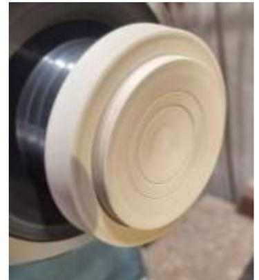
6. Using the lid as a sort of loose fitting jam chuck, mount your box section onto the lid tenon and hold firm with your tail stock. Align the grain as best as possible and turn to finished size & shape. Sand when completed.
