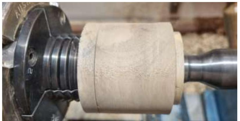
7. Remove the lid section from the chuck and mount the box section. If your chuck jaws do not fit into the box, you may need to use a jam chuck. Gently turn away the tenon and tidy the base of your box. Sand when complete. Your box is now complete.
