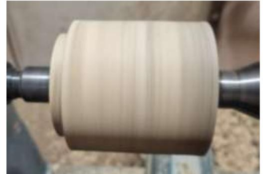
2. Mount into your chuck using the tenon. Cut a recess for your inlay into the end of your blank (lid) ensuring the sides of the recess are square and the bottom is flat. The recess should be around 5mm deep and 5mm – 10mm from the edge.
