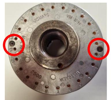
3. Remove the 2 pinion retaining pins and keep safe, then remove the 2 pinions by sliding outward from the chuck body.
