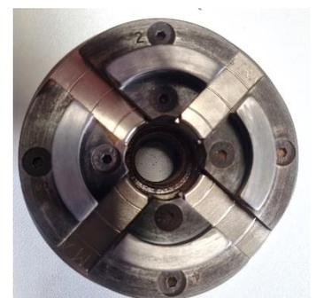
12. Replace the scroll into the chuck body. This bit can be a little fiddly as each jaw slide will need to be wiggled to get the scroll to seat properly. You will feel and hear the slides locate into the scroll as they find their home. Once seated properly replace the circlip.
