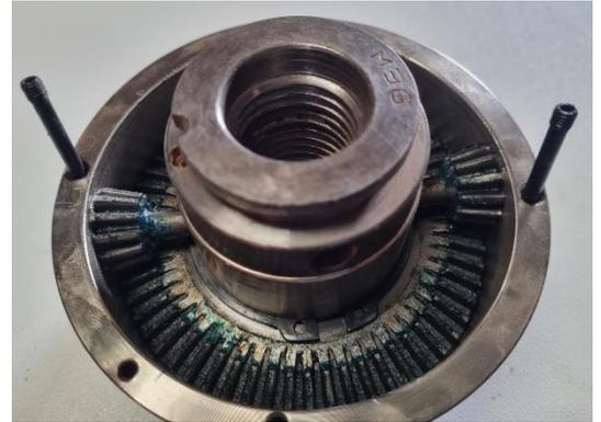
14. Using your finger put a blob of grease onto the tops of the pinions. You don't need to flood the area, but conversely don't use too sparingly. Do not use products such as RP7 or WD40 as they are too thin and what doesn't run away will attract dust. Also do not lubricate the jaw slides on the other side of the chuck as it will also attract dust and potentially stain any timber it touches.
