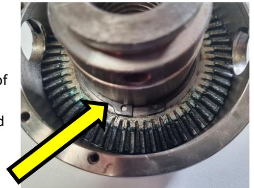
5. Once the circlip has been removed, you can turn the chuck over and slide the scroll out. The photo above shows the teeth that the pinions engage while the picture to the right shows the scroll gear that the jaw slides work against.
