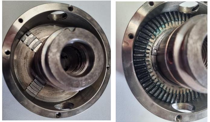
13. Replace the pinions and pinion retaining pins. You may need to rotate the pinions slightly with the chuck key (allen key) to get them to locate properly. The retaining pins do not need to be overly tight as the backing plate will help hold them in place.
