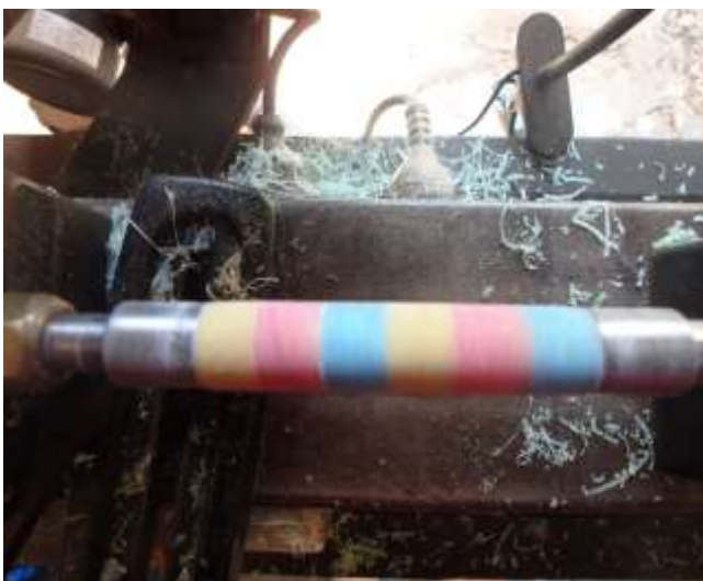
After normal sanding 180 to 600 grit
