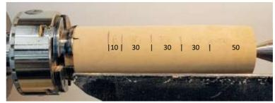
Hollow out the end of the blank to form the internal bowl of the goblet approx. 45mm in depth. Sand and finish at this time.
