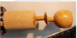
Loosen chuck and move goblet lip 10mm away from tool rest. (This is 180 deg from the previous offset movement)
