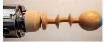
Support goblet cup with tailstock. Sand and finish. Part off to complete.
