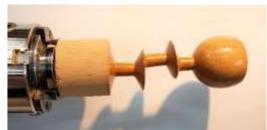
Loosen chuck and reseat goblet flush to chuck jaws. Shape goblet base and using a parting tool undercut the base, leaving approx. 15mm.
