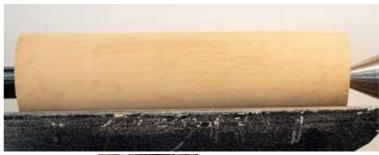
Cut a tenon 10mm in width on one end to mount in your chuck.
