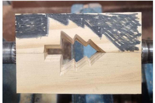
9. Again using high speed on your lathe, remove the unwanted sections from your blank.
