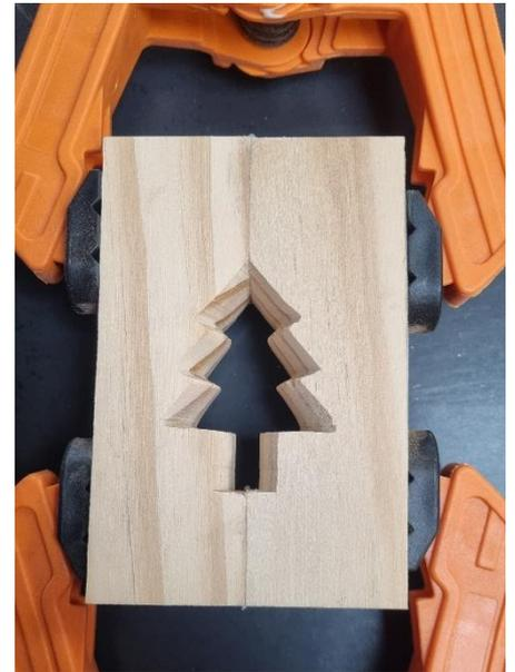
7. Glue and clamp, ensuring the internal design is aligned properly
