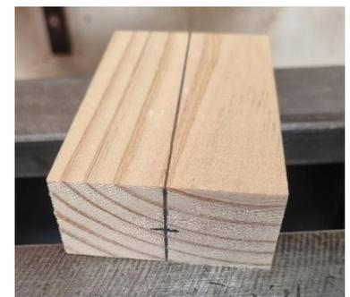
3. On one face of your blank on the upper edge, draw half of your pattern and colour in as shown in the photo. This will allow you to see your pattern while the timber is spinning, making it easier to know what areas to remove.
