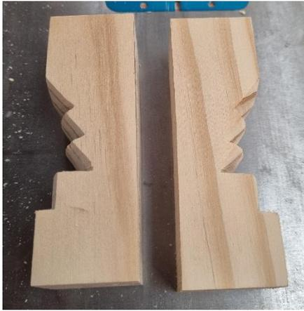
5. Remove from the lathe and cut in half along your marked line
