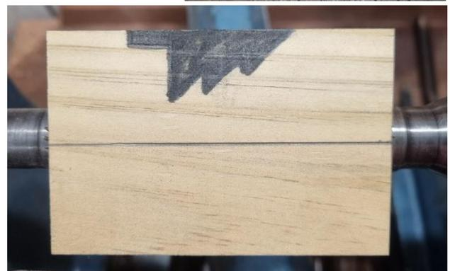
4. Turn away your coloured in pattern. Using the lathe at high speed will make the job easier, as there is less time between the timber making contact with your chisel and your pattern will be more visible.
