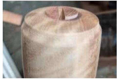
Cut a thin wedge from the same timber as the mallet head and glue into the handle slot. Hammer it in gently to knock it in tight.
