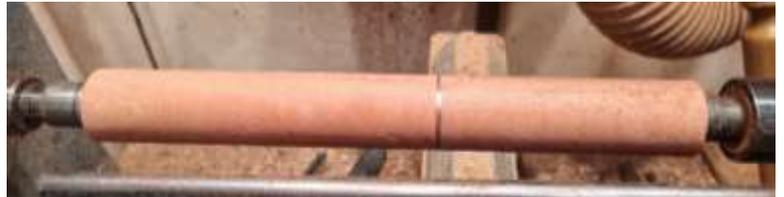
Turn down the marked section to form a long tenon that will fit into the mallet head. It does not need to be an overly tight fit, a snug fit that can be pushed on by hand is ideal.
