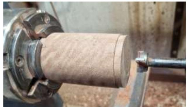
Remove the blank from the chuck and mount a small piece of scrap wood. Form a short tenon to suit the hole in the head blank. Using a cone live centre in the tail stock, remount the head between centres.
