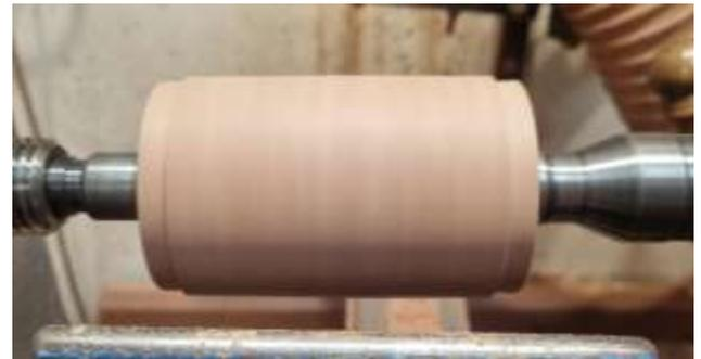
Mount your blank in a chuck, ensuring it is centred. Using a 25mm forstner bit or similar mounted in your tail stock, drill through the centre of your blank. If you can drill all the way through from one end, take care not to drill into your chuck. If your drill bit is not long enough to go completely through from one end, drill as far as possible and reverse the blank in the chuck and complete the hole from the other end.
