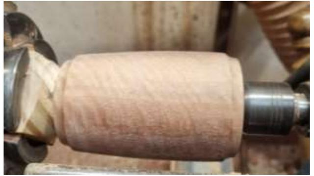
Mount the blank for your handle between centres and rough turn to round. Mark a line slightly longer (2-3mm) than the length of your mallet head.
