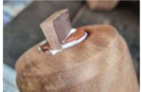
Once the glue has fully dried, carefully cut off the overhanging wedge and handle protruding from the mallet head and sand smooth.
