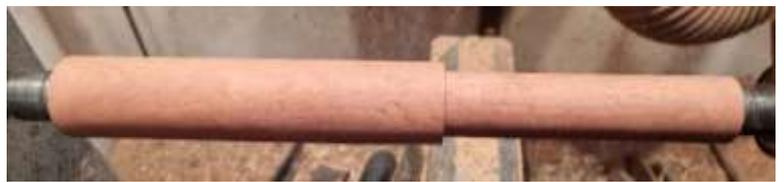
Test fit the head onto your handle, ensuring that the handle pokes slightly through the head. Adjust your handle if necessary.
