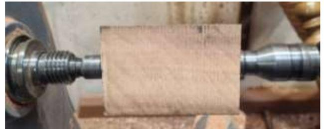
Rough the blank to round and create a tenon on each end to allow for mounting in a chuck. Don't be too concerned with the shape of the head at this stage, as we will remount it later to complete.
