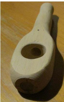
Bore a hole, say 20 mm in diameter, across the handle near its mostly unshaped end, to accommodate the cord around the stem.
