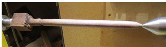
but strong enough to withstand a bit of rough treatment, perhaps with a small cross-wise hole drilled in it. Taper the end near the tailstock to a blunt point, to take a small nail or pin in the centre point to reduce wear –the greater mass of a larger top creates more wear on the point, so some
