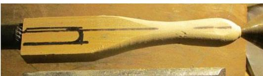
Turn a handle from, say, pine board or something fancier, 130-150 mm or so long x about 30 mm wide x 19 mm thick (i.e. with a rectangular cross-section), held between centres. If you are to make a horizontal handle, set the turning axis a few mm off the centre line of the piece to give more
