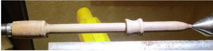
The stem can be made a greater diameter where it passes through the base – enlarge the hole in the base to accommodate it if needed. Allow enough length below any boss to accommodate the base and to allow the top to tilt by perhaps
