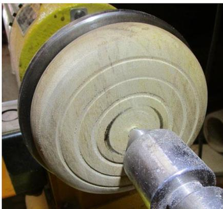
You can leave the edges of your disc square to the face, or shape them however you like –making the edge very thin may be unwise, because the spinning edge may then bruise anything it hits, or even break off. Keeping the edge broad increases the mass of the base out towards the edge, and the moment of inertia, which aids the duration of spin considerably. Shape a cross-section for the base however you like, also keeping it thick enough at the centre to support the stem well.
