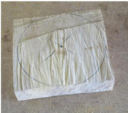
Select timber for the base that has a pretty uniform density across the plank, otherwise the non-uniformity may well induce out-of-balance forces when the base is spun –that is if you are after a wobble-free version, and want to avoid re-turning it or adding little weights to the rim to rebalance it.
