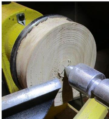
With the lathe on a lowish speed to start with, turn the base circular with a sharp gouge, parting tool, skew -whatever you are comfortable with. Face the disc if it doesn't run true with the faceplate. Flatten off any remaining wood at the centre with abrasives or a chisel.
