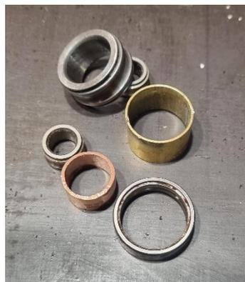
Using callipers, measure the inside diameter of your selected ferrule.
