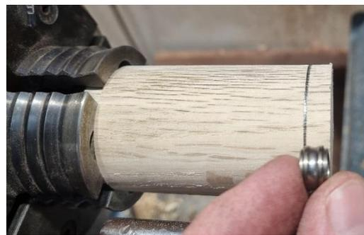
Using your callipers to measure, form a tenon to suit your ferrule. Use the line to dictate the tenon length, slightly longer is better than shorter.
