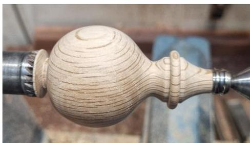
Using a fine handsaw, cut the remaining spigot from the end and sand to complete.
