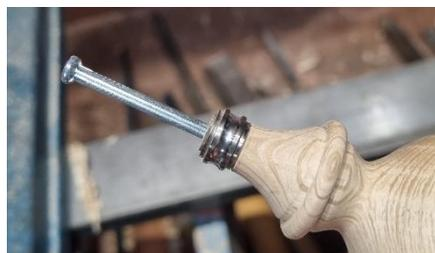
Using a grinder or file, grind a 3 sided point onto the end of your nail. This will allow it to cut as it is twisted.
