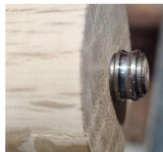
Remove the chuck from your lathe and using a cone tail centre into hole that you drilled earlier, remount the blank between centres.
