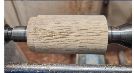
Mount your blank in your chuck. Using a drill chuck in your tail stock, drill a hole slightly smaller than the diameter of your concrete nail.
