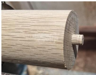
Remove the blank from your lathe and using a hammer, knock your ferrule onto the tenon. If the fit is too loose, wrap a small bit of masking tape around the tenon.
