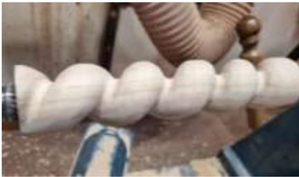
Moving onto abrasives, finish smoothing the piece, taking care to remove all tool marks and pencil lines. As a suggestion, using long thin strips of cloth backed sandpaper is much easier and faster than using smaller pieces.
