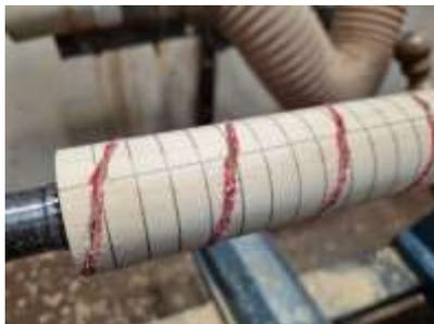
Using a fine-toothed handsaw cut along your diagonal lines. Try to maintain a constant depth, as these cut lines give your rasps and files something to follow and indicate how deep to go. It may help to stick a piece of tape along your saw to act as a depth indicator.
