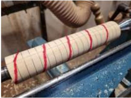
Mark diagonal lines to join the corners of the squares and continue around the spindle. With the double bine spiral, mark a second line opposite your first line. Indicated in green on the picture to the right.
