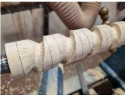
Using the principle discussed above to guide your cut direction, begin removing wood with your rasp or file using the saw cut as a guide. Orientate the timber and start from which ever end is more comfortable for you. Cut down to your saw cut depth.
