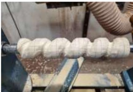
When you have completed roughing one side, flip the timber around and rough out the remaining side.
