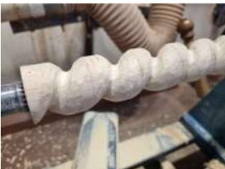
Using finer rasps or files, continue to refine and smooth the shape, try to ensure an even depth and radius on your bines.
