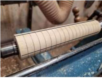
Set your tool rest at about centre height and draw lines along the spindle to mark the diameter into even quarters. Larger diameter projects will require more division lines, but keep them evenly spaced. If you are planning on a 3 bine twist, divide your spindle into thirds (or multiples of). See 'tips' at the end of this project sheet for help in doing this.
