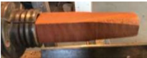
Mount a spindle blank with a diameter slightly larger than 25 mm in a suitable scroll chuck and reduce to round..
