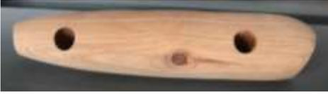
Shape the nose and rear of the body as you wish. This can be done on a linisher, belt sander or using a file etc. Apply the finish of your choice.
