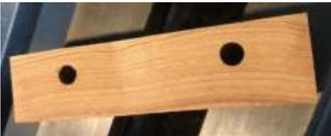
Determine the diameter of the dowel to be used as axles, in this case it was 12.7 mm. Drill two holes slightly larger than the axle diameter 50 mm in from both ends and 20 mm from one edge as shown in the photo.
