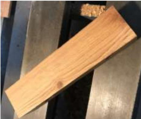
Select a spindle blank approximately 200 mm long by 45-50 mm square. At least two faces need to be at right angles to each other; use these faces to ensure drilled holes are perpendicular to each other. Accurately locate and using an awl or other suitable tool mark the centres of both ends.
