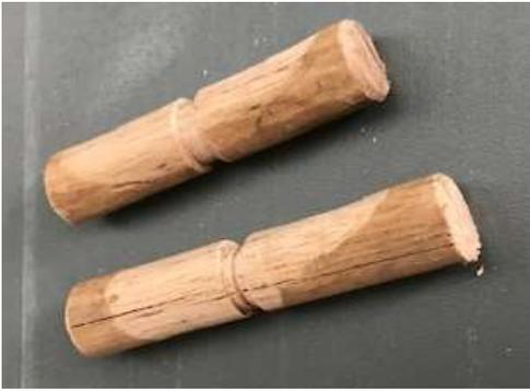
Axles are simply pieces of dowel cut to length. Length is determined by a trial and error process ie cut over length then fit wheels and axles to car body and keep reducing the length until it looks right.
