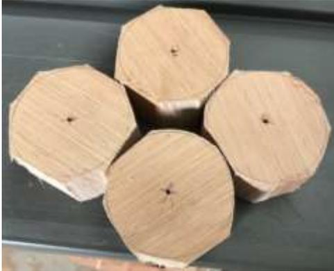
Prepare four wheel blanks of approximately 50 mm diameter. Thickness is up to you. The ones in the photo are 32 mm thick – one was cut in two to produce narrower front wheels.
