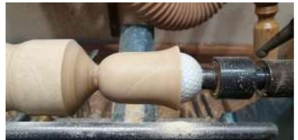
9. Begin shaping the goblet's stem from the bowl toward the chuck. Keeping the remaining blank as is, thin down in sections to your finished diameter, approximately 25mm at a time works well. This maintains as much strength as possible to the stem section. Once completed, gently sand and part off (below right)
