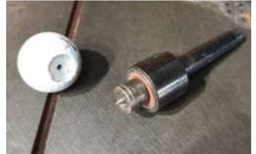
8. With the tail stock gently pushed up, finish the shaping of the outside of the bowl section.
