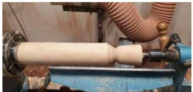
5. With the tailstock out of the way, begin hollowing. If you have a 3 point steady, it will make the job much more stable. To make hollowing easier you can use a drill or forstner bit to remove the bulk of the wood. As you will be hollowing into end grain, remember to take it slowly and make light cuts
