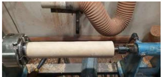
4. With the tailstock still in place to provide support, begin shaping the bowl of your goblet, only rough out the shape at this stage, as it is better to finish it after you have completed the hollowing. When you are happy with the rough shape, remove the tailstock.
