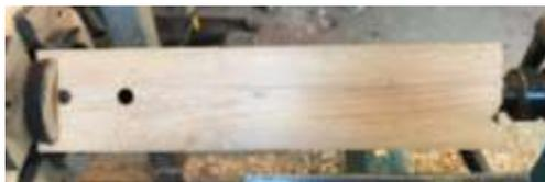
Use a roughing gouge to reduce the blank to a cylinder.
