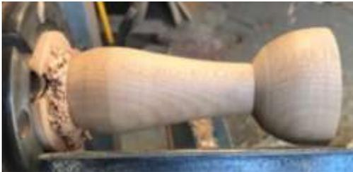
Shape the rattle section to match your hollow or design of your choice. Remember to make the walls thin enough that the sound will transmit through them without being so thin that they are likely to break.
