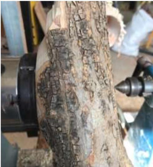
Mount the blank in your scroll chuck and bring up the tailstock for support.
