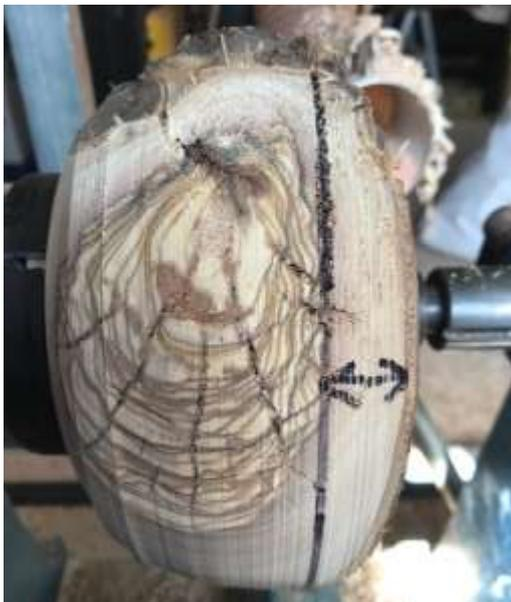
Use pull cuts from the headstock and tailstock ends to reduce your blank to a round. Cutting against the grain using gentle pull cuts from the tailstock end are needed to avoid bark separation and or splintering of the trailing edges of the cut. The black line is the point on the bowl where the entire circumference will be cut by the gouge. The arrow indicates the area where cutting against the grain produces best results. Remember be gentle – no aggressive cutting here please.
