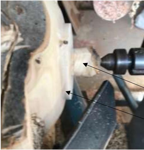
Use a bowl gouge to produce a tenon to suit your scroll chuck. Leave a substantial spigot for the live centre support because if this fails the blank will come off the lathe.
