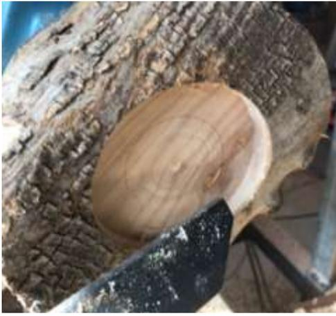
Remove the tailstock support.
