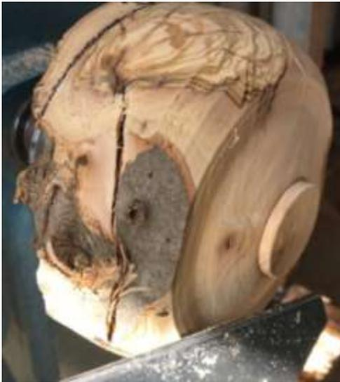
Refine your tenon. Here you can see the tenon has been reduced from approx 85 mm to 50 mm to suit another scroll chuck as the original tenon was out of proportion to the likely diameter of the finished bowl.
