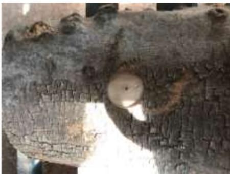
Use a Forstner bit or some other method to ensure your drive centre can achieve a good grip on the timber. This should be in the centre of what will be the top of the bowl. If you don't do this the blank is likely to be thrown off the lathe and could result in injury to you or property damage.
