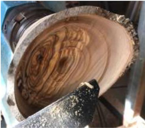
Decide on the wall thickness and continue hollowing in small sections. It is difficult to come back to work near the rim as you go deeper as chatter will occur and distortion of the walls is possible during the turning process. Use calipers to ensure an even wall thickness. Once again the use of a freshly sharpened scraper can assist with surface finish.
