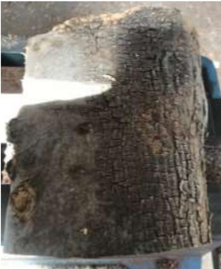
Select a piece of branch wood approximately 180 mm diameter and 200 mm long. Branch wood often has one side flatter than the other due to stresses associated with gravity. If your blank has this characteristic consider making the flat side the top of your bowl. This will allow you to achieve a much flatter rim to your bowl and is easier to master for your first natural edge bowl.
