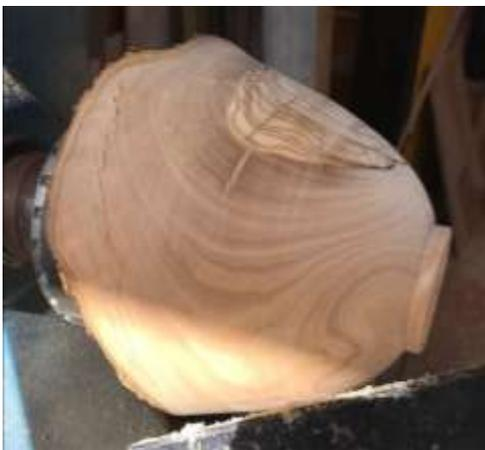
Refine the outside shape of your bowl. The photo shows a bowl with an asymmetrical ogee profile. A traditional or negative rake scraper can be used to remove ridges left by the bowl gouge.
