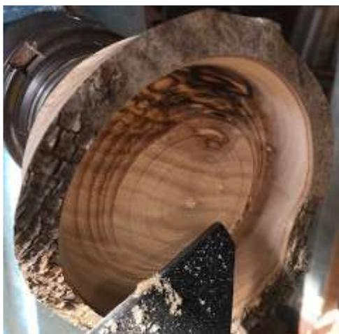
Mount your bowl in the scroll chuck using the mortice and commence hollowing out your bowl. A bowl gouge is recommended as carbide tipped tools are usually scrapers and can damage the bark / rim. Present your gouge to the work with the flute fully closed ie the gouge is on its side and rotate slightly to produce the cut. Once again be gentle.
