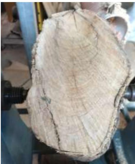
Mount between centres with the top of the bowl toward the headstock (you can clearly see that this surface is flatter than the other side. I prefer steb drive centre and a cone live centre.
