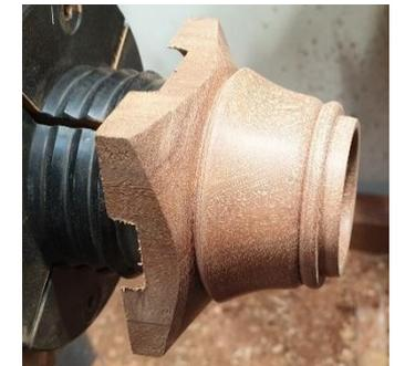
10. Using a scrap block mounted in your chuck turn a jamb chuck to reverse mount the base section. Use the tail centre to hold the base onto the jamb chuck (not pictured)
