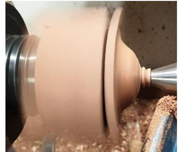
8. Remove the tail stock and very gently complete the centre of the box lid as not to break it from the jamb chuck. Gently sand as required. Once complete, remove the lid from the jamb chuck. If the lid is a tight fit it is advisable to use a knife and gently prise it loose as the corners can be fragile at this point.
