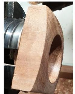
6. Remove the lid section from the chuck and mount the base section using the recessed tenon. Turn a short tenon on the base to accommodate the hollow on the lid section. At this stage make the tenon a tight fit to act as a jamb chuck.
