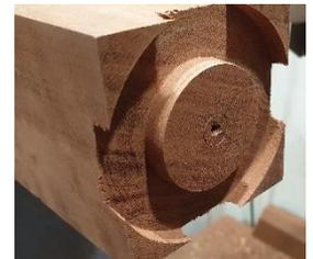
4. Take the blank off the lathe and mark a line to delineate the lid from the base of the box. Work on about  $\frac{2}{5}$ th of the total length for the lid and cut on a bandsaw. Do not part off on the lathe as it is highly likely that the corners of the blank will get damaged
