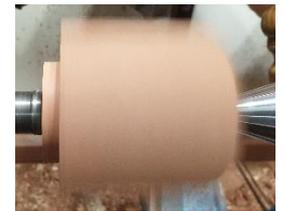
3. Mount the blank in a chuck using the tenon. Turn a recessed tenon in the base, take care to leave the outer corners to be used as feet.
