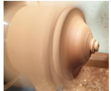
9. Shape and hollow the base section and sand as required. At this stage it is advisable to sand the tenon that the lid sits on to make a slightly loose fit. When removing the lid people tend to hold the lid corners and having a tight or press fit may result in breakage. Remove from the chuck
