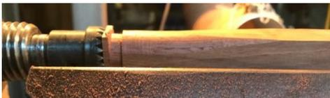
Use a parting tool to form a groove approximately 10 mm from each end of the blank. Diameter is not important as long as the groove is down to round.
