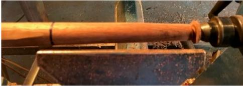
Mark the length of the blade (from the tailstock end). In this case it is 130 mm.
