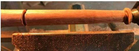
Use a parting tool to define the transition point between the handle and the blade. In this case it is approximately 10 mm diameter.
