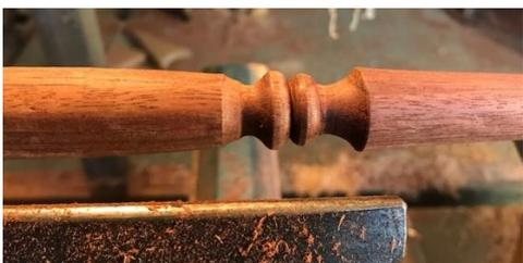
Double bead transition completed. Note that the beads are intentionally different diameters, identical beads do not work in my opinion.
