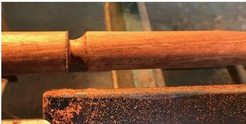
Create a flowing curve for the transition as shown. Make sure the curve is continuous.
