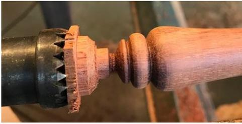
Part off using the skew chisel working through small cuts toward the headstock. This method minimises torn grain and makes sanding the knob much easier.
