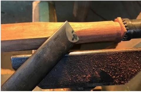
Use the skew chisel to reduce the blank to a cylinder. Note that the cut is occurring at the quarter point of the cutting edge as shown by the arrow.
