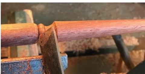
Use the skew (or other tool of your choice) to create one or two beads to define the end of the handle. You can use the short or the long point of the skew but care needs to be taken to present the skew at the right angle or a catch will occur.
