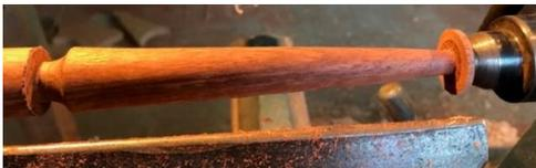
Taper the blade section from the high point of the transition to the tailstock end leaving an approximate diameter of six mm. This section does not require sanding as it will be worked on at a latter stage.
