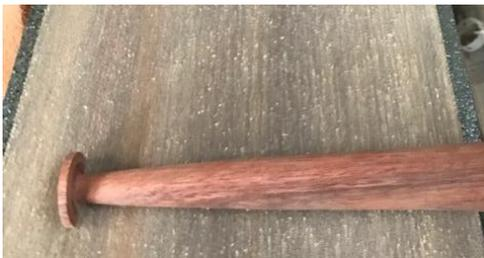
Use a linisher/belt sander to reduce one side of the blade to a flat. Take into account grain orientation to maximise strength. Take care to not damage the transition point by over sanding. Note that the sanding is being done on that section of the belt where there is virtually no gap between the edge of the belt and the edge of the linisher.
