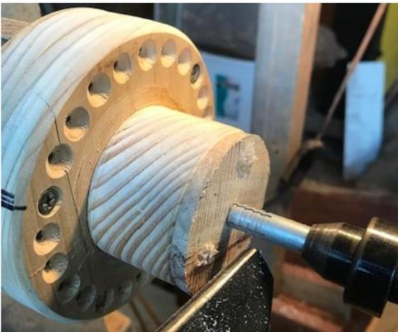
Place a piece of non-slip matting or paper towel between chuck and sanded surface of the pendant and secure with a live centre extender to create a friction drive.
