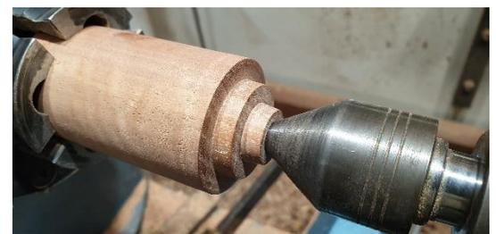
11/ Put the cover section on the base and hold in place with a live centre. As earlier, mark the depth of the hollow to prevent turning through the cover.
