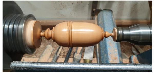
13/ Sand the tenons of the base section to make a slightly loose fit for the thimble and cover. Finish if required. Part off.
