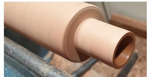
4/ Decide on the size of the cover section and part off. Remember that the cover will need to go over the thimble and still have the depth to sit on the tenon on the base.
