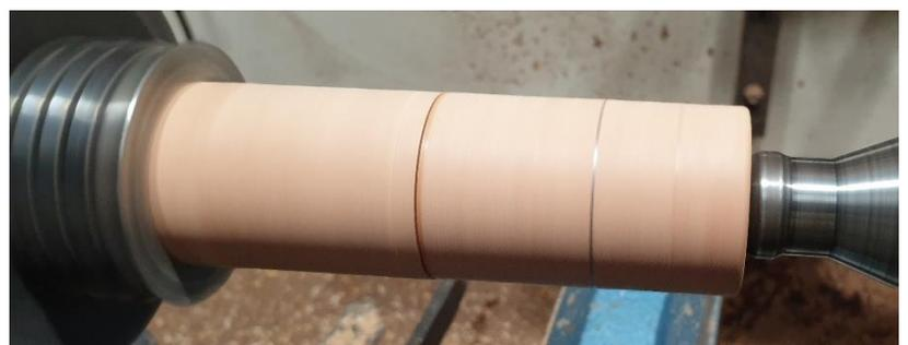
12/ Shape as desired. Sand and finish. Part off the cover section and remove.
