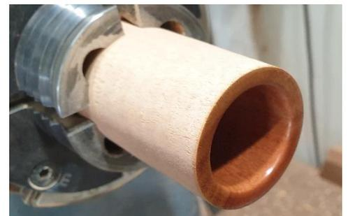
10/ Remove the cover section from the chuck and remount the base. Using a cone live centre in the tail stock to align the needle hole will make centring much easier.
