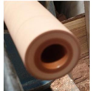
3/ Measure the depth of the hole and add about 5mm and turn down the outside of the thimble. Don't get too concerned with the finished shape at this point as we will remount it to finish it off later. Part off when complete.
