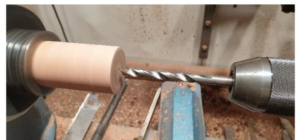
6/ Turn a tenon on your base section to use as a jamb chuck for your thimble. Measure the depth of the hole in your thimble and mark a line. Mount your thimble.
