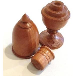
1/ Begin with a timber blank approx. 45mm square and 170mm long. Mount between centres and turn to round, then mount into a scroll chuck.
