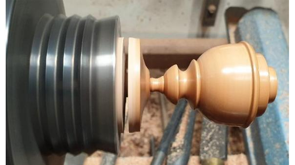
14/ Reverse the base section in the chuck to finish the bottom. Another jamb chuck may be required if your chuck jaws are too large. Sand and polish.
