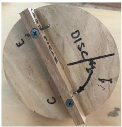
The photo shows the rear of the completed chuck with the concentric and eccentric points marked along with the location of jaw 1. Always remounting your eccentric chuck in the same position on your scroll chuck aids accuracy when multipe facets are being turned.
