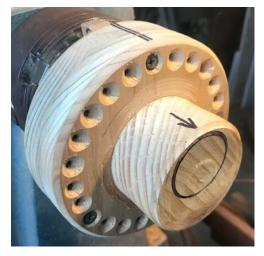
Move the chuck to the eccentric position and mark a circle on the face of disc 2 with a point tool or long point of a skew. Use a permanent marker or other method to mark the point where there is the shortest distance between the circle and disc 2 (in this case marked with an arrow). This aids aligning blanks to cater for grain direction / timber strength etc.
