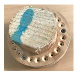
Drill and countersink holes to match your screws. Fasten disc 3 to disc 1 using the three remaining screws at equidistant centres. True up the face of disc 3 taking care not to contact the screw heads.
