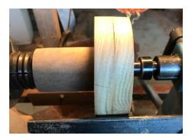
Drill a small (1 or 1.5 mm) hole in the centre of discs 1 and 3. Use a relatively loose fitting nail or similar in the holes to ensure discs 1 and 3 are aligned then place discs 1 and 3 against the jaws of your 4 jaw chuck or waste block (as shown) and secure by tightening the live centre (ring centre works best) to create a friction drive. Turn the discs to a cylinder; don't bother to square the ends.
