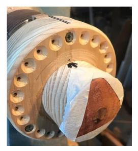
This chuck can be used in the making of pendants and boxes etc where offset or multi sided forms are desired. Blanks can be attached using hot melt glue, double sided tape or masking tape. The chuck can also be easily adapted to a screw chuck by gluing in a screw to the centre of the sacrificial disc (see below for a description of the parts).
