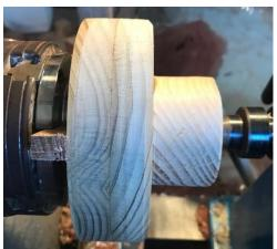
Mount the assembled eccentric chuck onto your 4 jaw chuck in the concentric position and true up the sides and face of disc 2.
