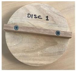
Cut the cross piece to match the diameter of discs 1 and 3. Glue and screw the rectangular piece of wood accurately across the centre of disc 1. When the glue has dried true up the disc. Drill an interference fit hole toward the outer edge of the cross piece where jaw 1 and the cross piece intersect then insert one of the nails (not shown) – ensure it is a tight fit – if not use CA glue to hold it in place. Cut off the point of the nail.
