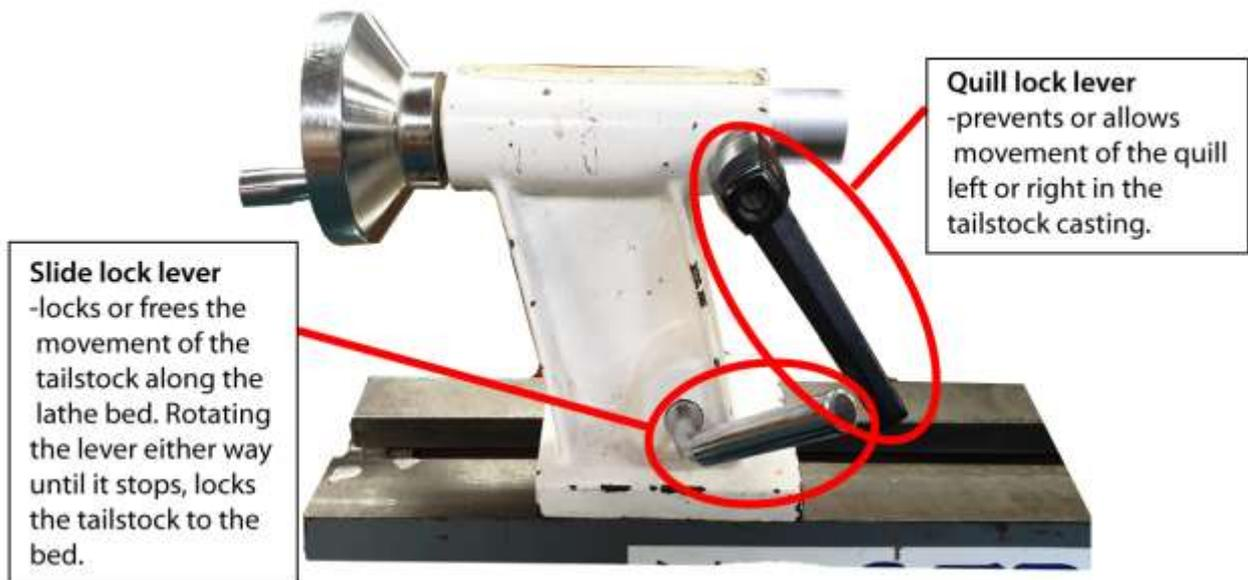
Winding the quill all of the way towards the rear ("retracting the quill") generally ejects anything inserted into the spindle. But if a live centre or drill chuck becomes jammed in the quill, a "knock-out bar" can be used to remove it.
