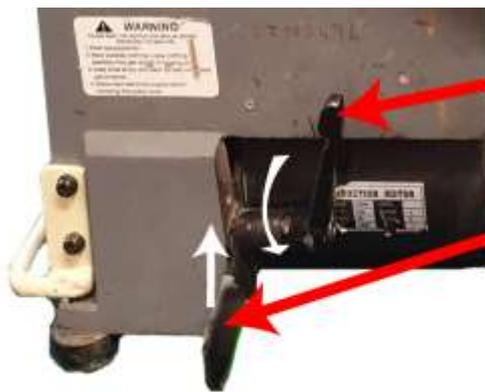
1. Locate this locking clamp below the headstock and loosen it by rotating the handle downwards from the position shown.
