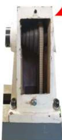
Back view of headstock with safety cover removed showing the spindle pulleys and drive belt position giving the slowest spindle speed.
