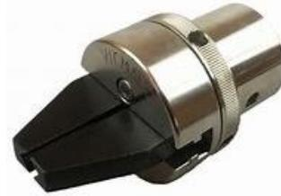
**Vacuum chucks** Vacuum Chucking systems have been designed to aid in Woodturning. It enables an item to be re-mounted on the lathe for finishing without risking further holding marks. Rotating Unions are designed to enable the lathe spindle to turn freely whilst the hose and connection remain stationary.
