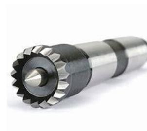
**Live centres** Used to align and support the workpiece from the tailstock end of the lathe. These centres are usually mounted on a Morse taper 1 or 2 stub. The section of the centre which engages the workpiece is mounted on bearings which allows it to spin freely supporting the wood without undue friction being generated.
