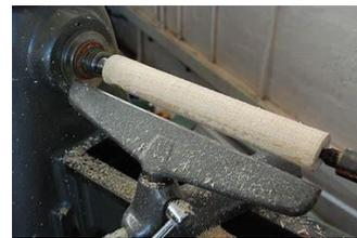
**Drive centres** Used to transfer the rotary motion of the lathe to the work piece (blank).
