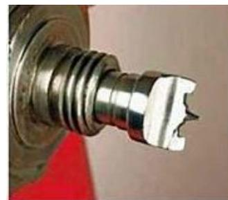
4 prong This centre has four driving prongs to engage the blank usually resulting in better grip on the workpiece. Once again it has a centre spur to assist with accurate alignment.
