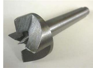
Safety The safety centre relies on the friction forces associated with the outer ring contacting the workpiece. The centre spur is often spring loaded and in some cases the tension can be adjusted. The benefit of the safety centre is that if a catch occurs the workpiece will spin without damaging the work. Not usually suitable for irregular shaped blanks.
