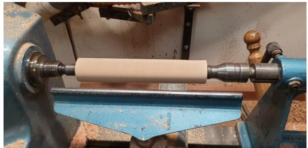
2. Turn a tenon 50mm long and about 25mm in diameter on one end, this will be the section that holds the blade.
