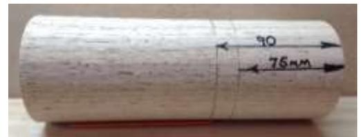
4/ Reverse the blank and mount into a chuck. Drill a 38mm hole, 6mm deep into the bottom, then a 34mm hole a further 4mm deep. Then a 26mm hole  $\frac{3}{4}$  of the depth of the base section of the blank.
