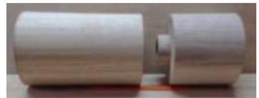
6/ Mount the top section into the chuck & drill a 20mm hole, 2mm deep, then a 7mm hole completely through the top section. Turn the tenon to fit snugly into the 34mm hole that is drilled into the top of the base section.
