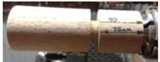
5/ Reverse the blank and mount on pin jaws, pin chuck or jamb chuck. Drill a 7mm hole  $\frac{3}{4}$  into the top of the mill, then part off the top leaving the tenon attached to the top. Drill a 34mm hole into the top of the base section 1mm longer than the tenon. Drill a 26mm hole through the rest of the base to meet with the previous hole. Remove steady rest if used.
