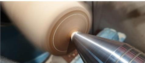
Insert the lid and hold in place with a tail centre. Shape the lid and blend into the top of the pot. Sand if needed.
