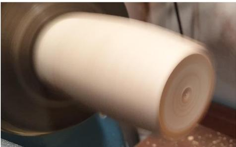
Reverse mount the pot using internal chuck jaws or a jam chuck and shape and clean up the bottom. Use the tail centre for support if required.
