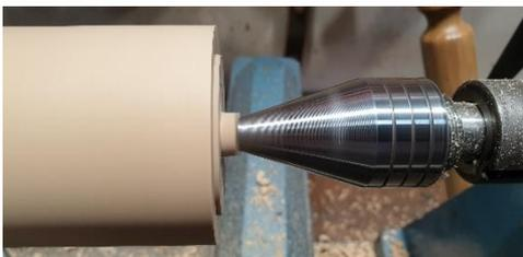
Make a narrow tenon on each end. This tenon is a depth guide, not for mounting in a chuck, so it only needs to be 2-3mm thick
