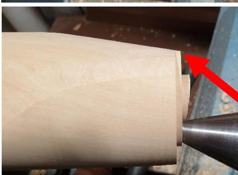
As the blank is now off centre, spin the blank by hand to ensure it clears the tool rest and adjust if needed. Ensure the blank is held tightly between centres. As the blank is now off centre you may need to adjust the lathe speed to minimise vibration. Begin turning. Make gentle cuts and allow the wood to come onto the tool. Turn the blank down to the depth guides at each end (indicated by the arrow). Sand if desired, be aware sanding will round the edges between the faces.
