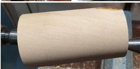
Remount the blank between centres, using the new points. Mount the headstock end to point 1 and the tailstock end to point 2.
