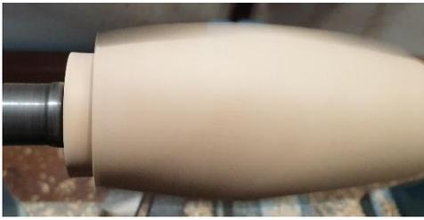
Remount the blank using the final set of points – headstock end at point 3, tailstock end at point 1 and turn down to the depth guide
