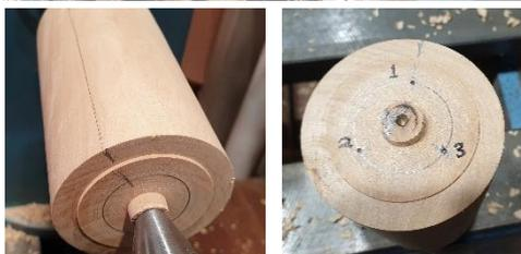
Draw a line along your blank and continue the line down the sides onto the 'offset circle' on each end. Equally divide the circle on each end and number, ensuring that the numbers match up on each end. Marking the points with an awl makes locating the centre easier.
