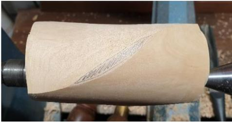
Once you are happy with the finish, remount the blank. Headstock end at point 2, tailstock end at point 3 and turn down to the depth guides at each end. If the depth guides are not deep enough a flat spot along the border between the 2 faces will appear (shown in the shaded area). Remount the blank to true centre and lower the depth guide tenons and repeat the turning process on the first 2 faces.
