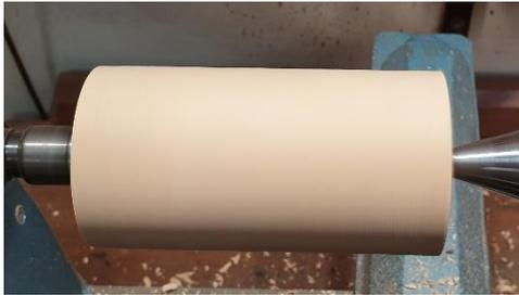
Turn a cylinder and square the ends. Make the waste around the drive and live centres as small as possible to reduce interference with the centres when remounting later.
